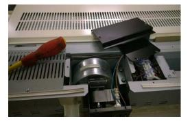
Access the drum between the drum casing and the heater body
